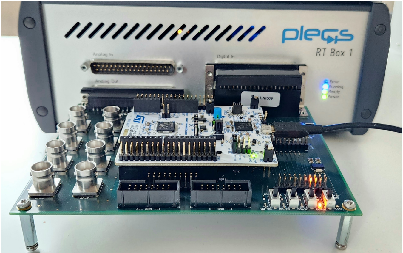
Figure 6: RT Box and STM32 Nucleo board via the Interface board
