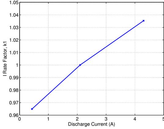
Fig. 5: Discharge rate factor  $k1$  vs. output current.
