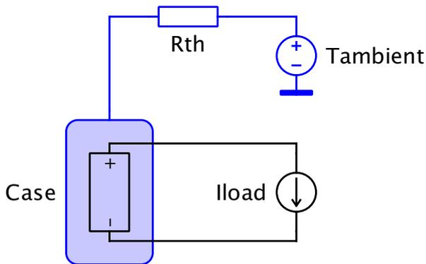
Fig. 7: Thermal circuit showing the heat flow path between the case (heat sink) and environment ( $T_{ambient}$ ). Multiple terminals can be added to the heat sink for modeling multiple thermal paths in battery pack applications.
