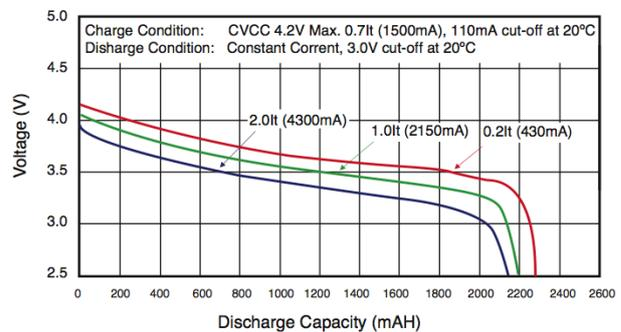
(b) Effect of load current on cell capacity (final SOD).
