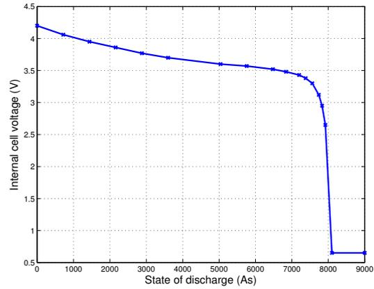
Fig. 4: Data points for modeling reference internal cell voltage,  $V_{cell\ ref}$ , as a non-linear function of SOD. Reference operating point is  $T = 20^\circ C$  and  $i(t) = 2.15A$ .
