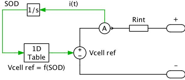
Fig. 2: Lithium-ion conceptual model.
