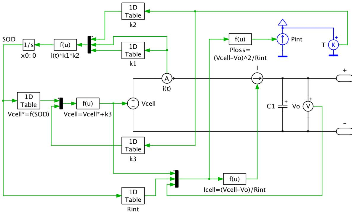
Fig. 6: Complete lithium-ion cell model. Internal losses,  $P_{int}$ , are automatically injected into the cell case.
