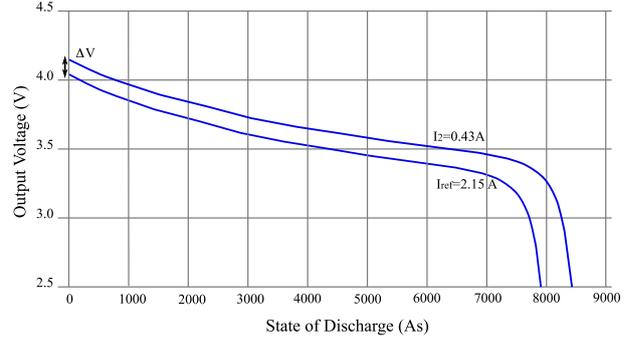
Fig. 3: Method for calculating of initial internal resistance,  $R_{int}$ , from datasheet output voltage curves.
