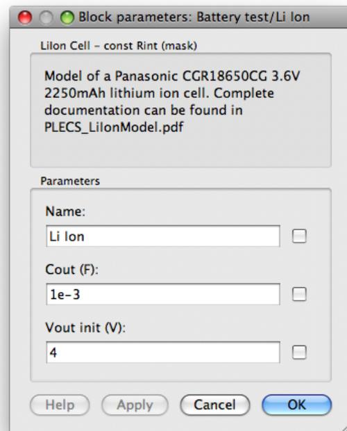
Fig. 8: Lithium-ion model parameters box.
