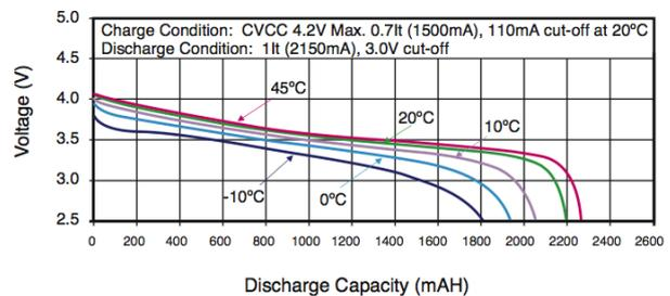
(a) Effect of temperature on cell output voltage and final capacity.
